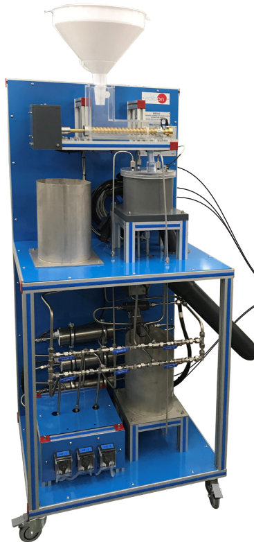
① Unit: UESLC. Computer Controlled Solid-Liquid Extraction Unit
